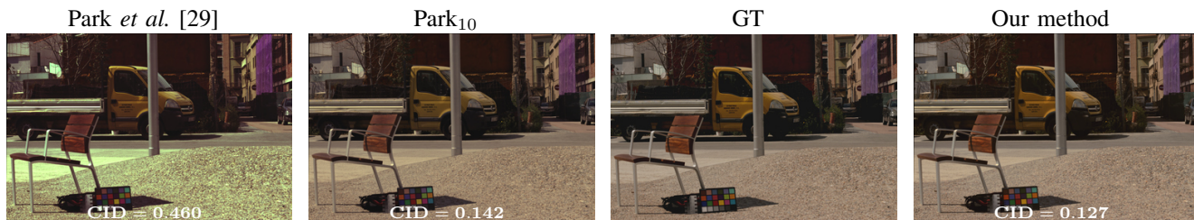
Fig. 6. Example of applying power 10 function to Park et al. [29]. The input images are a log-encoded reference and a gamma-corrected source. The first column presents the output of the original method from [29], the second shows the output of [29] applying power 10 (Park 10 ), the third shows the GT, and the last column shows our result.
