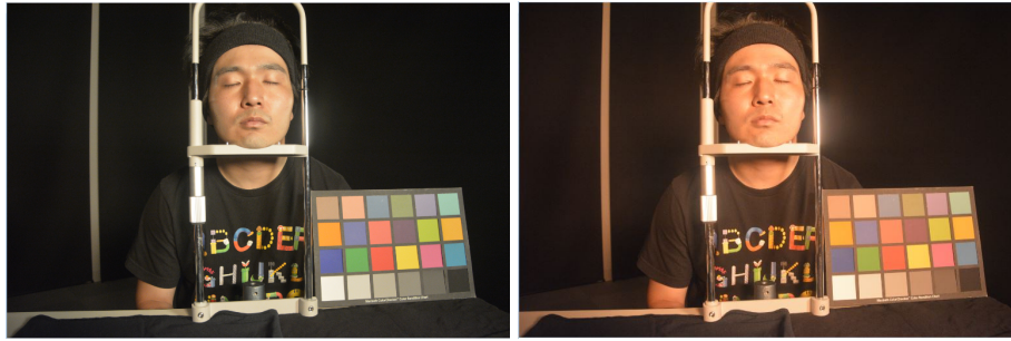
Fig. 2. Two images of the same scene from the dataset showing the ColorChecker chart, the left image is a normal capture and the right image was captured through a red filter, note that these 2 images are the camera pipeline outputs.
