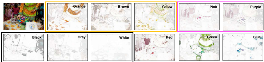
Fig. 3: Van de Weijer et al. [31] color naming method applied pixel-wise to the top-left image. The other 11 images show the 11 probability color names maps. Each color is displayed with a different map to aid visualization. Note that some linguistic color names share approximately the same hue and only differ in intensity— e.g., pink and purple . As tone curves are defined for all the intensity range we group: orange-brown-yellow , pink-purple , and white-grey-black . This grouping is represented by the boxes.
