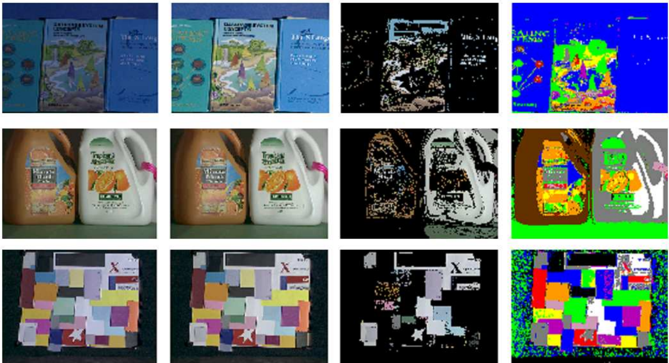
Fig. 5. Controlled indoor dataset. Original image (left), corrected image by proposed method (center-left), points weighting the selected illuminant (center-right), categorisation of corrected images (right)
