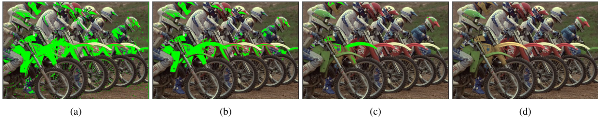
Fig. 2: Gradual mapping of colors. Out-of-gamut colors (in green) when (a): \gamma = 0 , (b): \gamma = -0.22 , (c): \gamma = -0.83 , (d): \gamma = -3.21 . As gamma decreases the number of out-of-gamut pixels is reduced.
