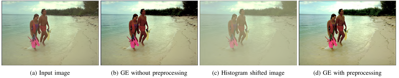
Fig. 7: Effect of preprocessing stage in GEA. Notice the trees in the background; the colors are preserved when GE is applied after preprocessing.
