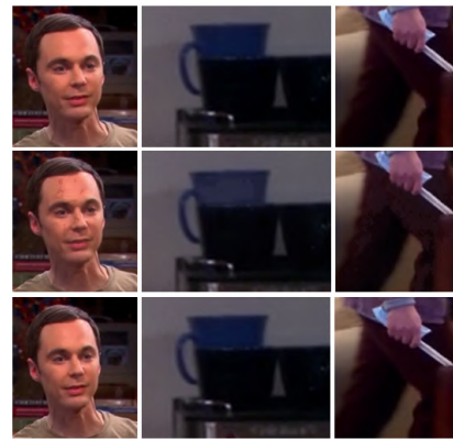
Fig. 14: Spatial artifacts due to GRA. Top row: original images. Middle row: effect of extreme target gamut. Bottom row: effect of realistic target gamut. The relationship of target gamut and spatial artifacts can be seen at the forehead of the person, cup and on the pants.
