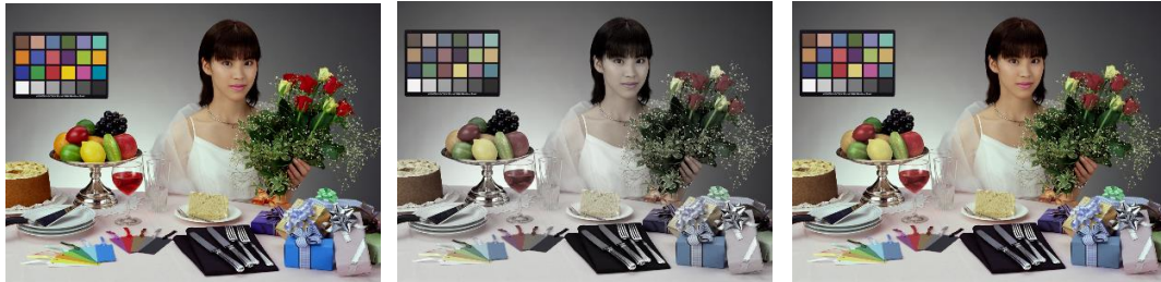
Figure 9. One-shot versus iterative GRA: a trade-off between quality and speed. Left: input image. Middle: output of one-shot GRA obtained in 0.58 seconds. Right: output of iterative GRA obtained in 1.47 seconds. It can be seen that the colors reproduced by the iterative GRA are more saturated than those of one-shot GRA.
